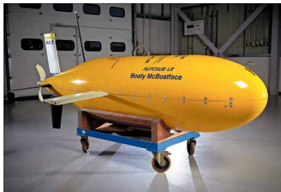
Boaty McBoatface - one of the National Oceanography Centre's autosubs - a long range autonomous vehicle that can travel for many kilometres and to great depths underwater, gathering scientific data. Photo: National Oceanography Centre (NOC)
