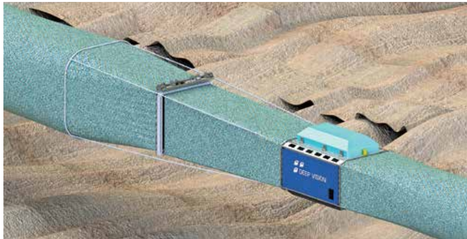
New technology such as the Scantrol Deepvision System is being used in ocean research. It takes photographs of and measures fish and invertebrates as they swim through the tunnel. There are only a few in operation at the moment and it can be modified to 3000m depth.
