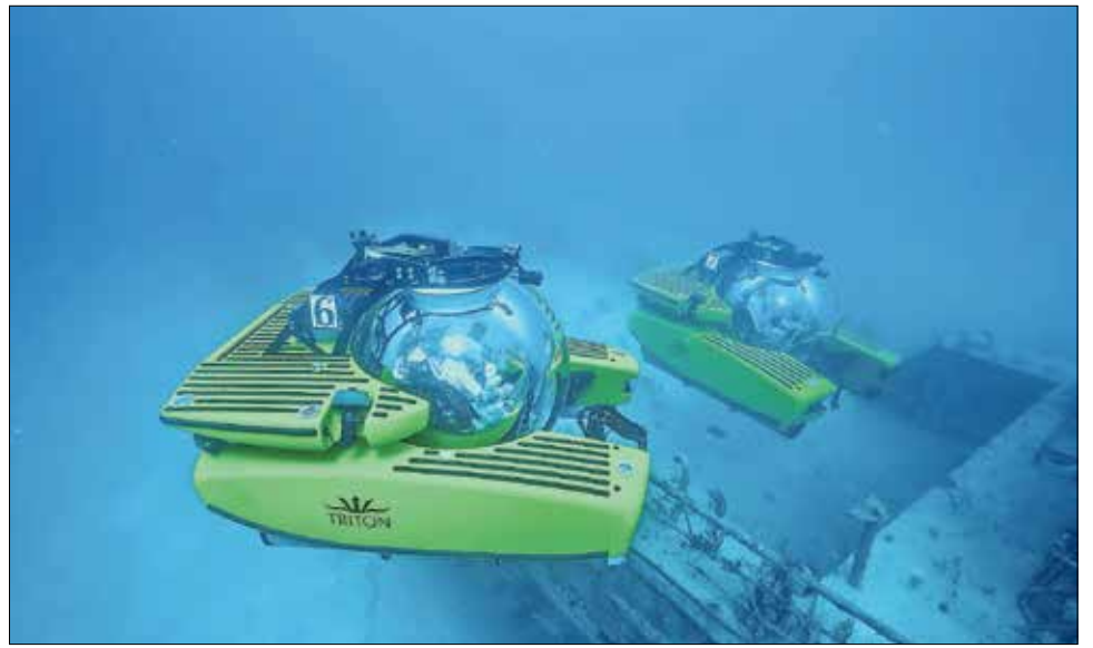
Triton: a three-person ocean research vessel with a diving depth of 2300m that will be used by researchers on REV I. Photo: REV Ocean
